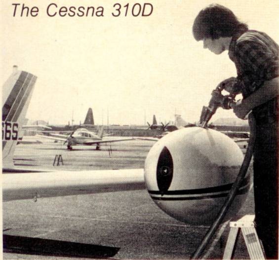
The two 51-gallon tip tanks on the 310D are the mains; with the addition of two 15-gallon auxiliary tanks a range of about 1,400 miles can be squeezed out of the airplane.
